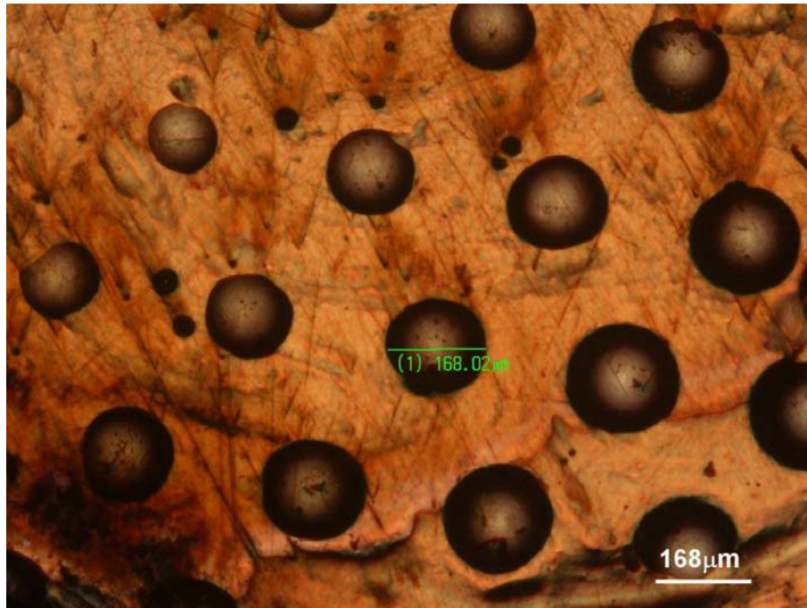
Figure 4.36 Replicated patterns by OM on the Au-based BMG materials imprinted at 177°C and 28 MPa for 10 min.
